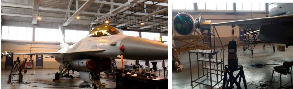
Figure 7: F-16 ground vibration testing measurement campaign. The right wing is excited by a shaker. Major part of the nonlinearities is related to the payload connection.
