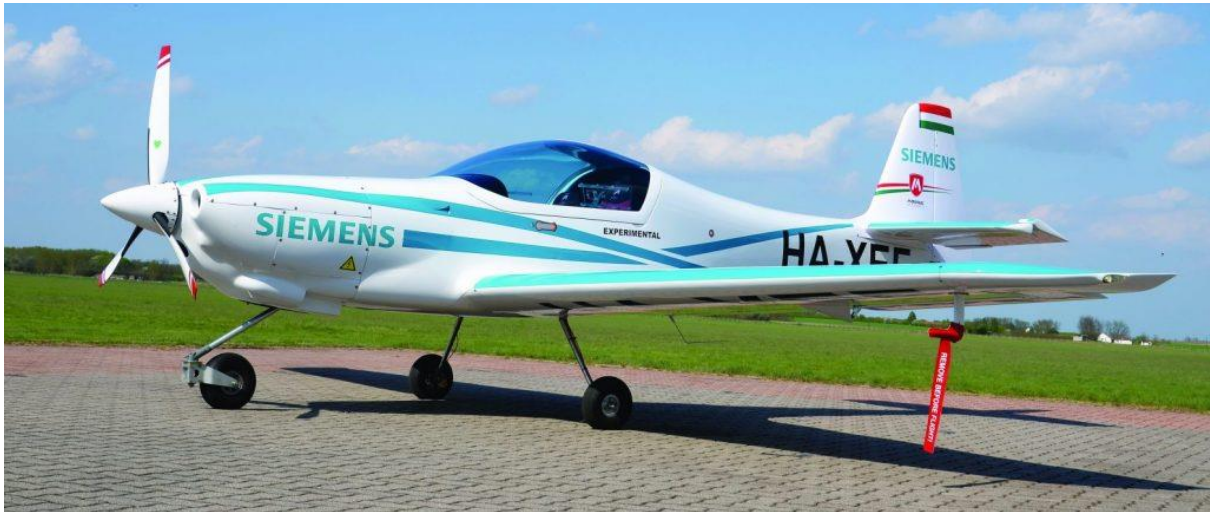
Figure 4: The eFusion battery operated small aircraft
