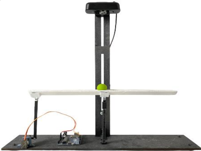
Figure 1: Ball balancing demonstration setup made up of a wooden base and stand.
